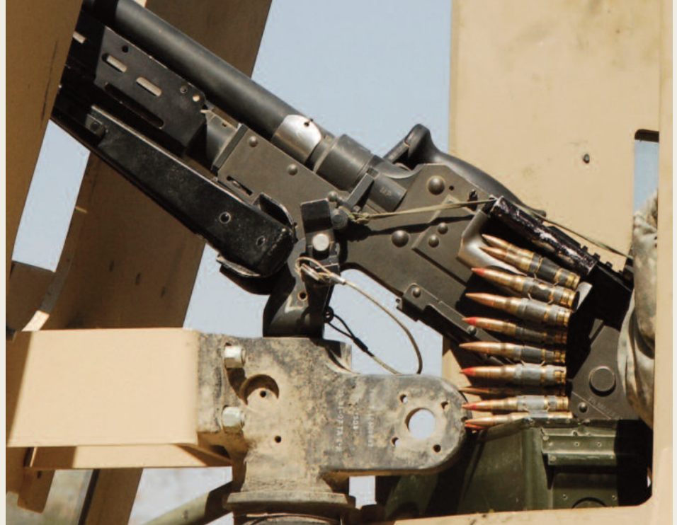
The Universal Pintal Adapter was made from ATI 425 ® -MIL Alloy for use with ARDEC's Objective Gunner Protection Kit (OGPK) and serves the purpose of mounting both the forward gun shield of the OGPK and standard weapons.
