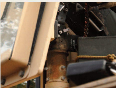
The use of ATI 425 ® -MIL titanium alloy instead of carbon steel to manufacture the Universal Pintal Adapter results in a 45% weight reduction for this component.
