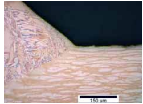
Figure 5: Micrograph showing no cracking of an AL 2003 weld after SSC / SCC testing
